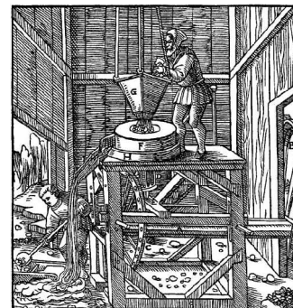
Figure 4: Grinding of ore with a water powered mill.
