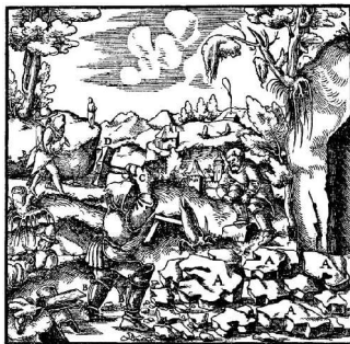
Figure 2: Crushing of the ore.
