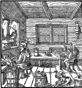
Figure 7: Handpicking at the sorting bench.
