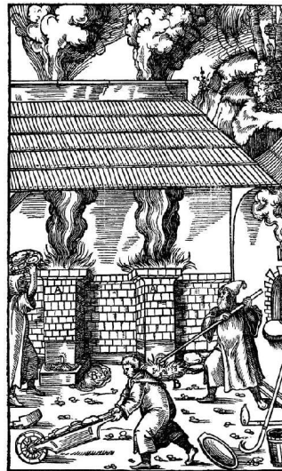
Figure 13: Smeltery with shaft furnaces in operation.
