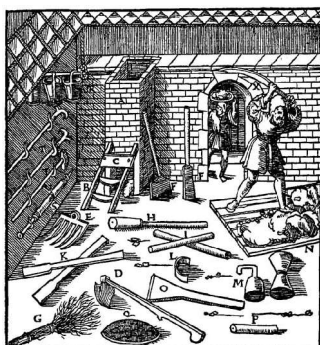
Figure 19: Tools for closing the front of a shaft furnace.
