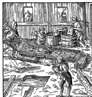
Figure 11: Washing on a table spanned with hides.
