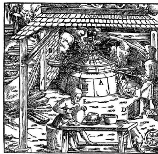
Figure 22: Cupellation furnace in operation.
