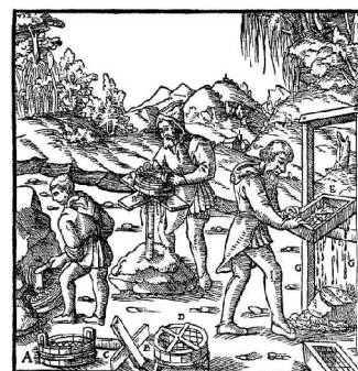
Figure 6: Three methods of screening ore.
