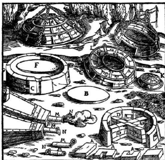
Figure 21: Construction of a cupellation furnace.
